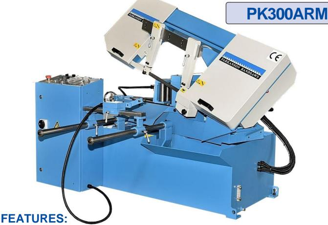
Fully automatic cutting with hydraulic power roller feed vice.
