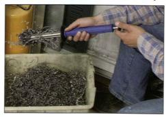
... and wiped off over the scrap metal container by actuating the mechanics without any risk of injury.
