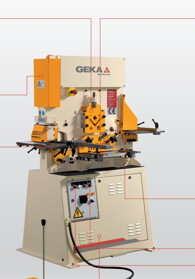
Shearing of flat bars up to 350x15 mm. Shearing of an L -leg at 45°
