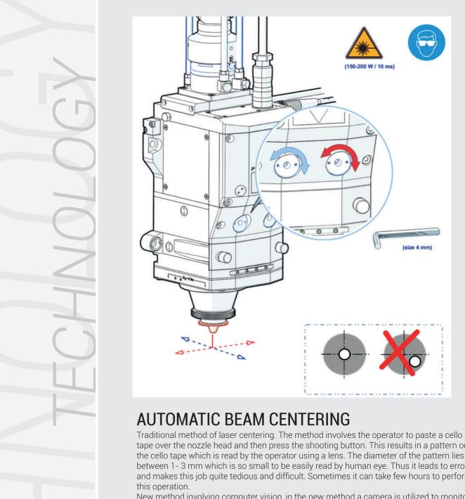
tape over the nozzle head and then press the shooting button. This results in a pattern on the cello tape which is read by the operator using a lens. The diameter of the pattern lies between 1-3 mm which is so small to be easily read by human eye. Thus it leads to errors and makes this job quite tedious and difficult. Sometimes it can take few hours to perform
