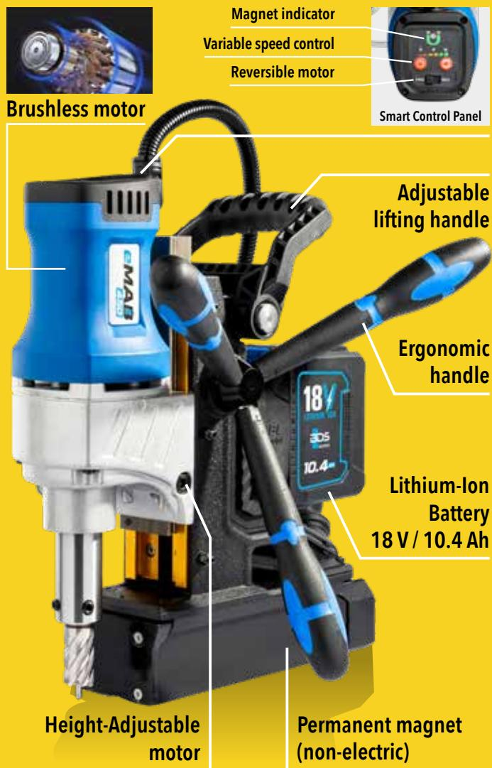
The new cordless magnetic core drilling machine with a 18 V / 10.4 Ah battery offers precise, cordless drilling for professional use. A brushless motor ensures high efficiency and low maintenance. The integrated permanent magnet provides strong adhesion and reliable performance – ideal for demanding applications on construction sites or in assembly work. It also features a reversible motor with clockwise and counterclockwise rotation for added versatility.
